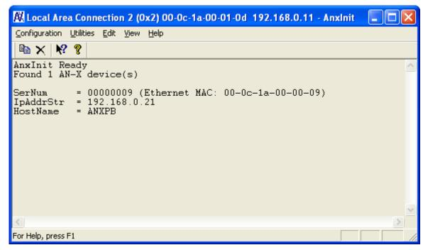
If AN-X does not find a DHCP server within about three minutes of starting up, it reverts to a temporary static IP address of 192.168.0.41 If AN-X is using this temporary IP address, it repeatedly flashes the SYS
