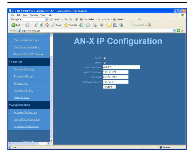
You can configure the AN-X to use DHCP or to use a static IP address.
