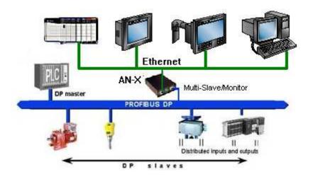
The AN-X-PBSLV communications module connects a computer or other device to a PROFIBUS network, using Ethernet.
