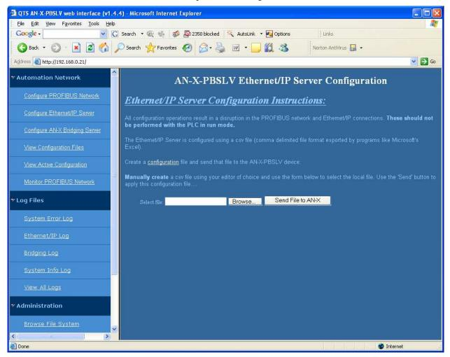
Type or browse the configuration file name into the *Select file:* area. Then click the *Send File to AN-X* button to send the file to AN-X.
