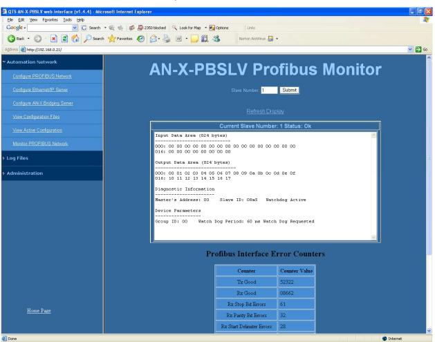
To use the web interface to view the current PROFIBUS network data on the AN-X, select Automation Network/Monitor PROFIBUS Network.
