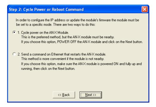
The preferred method is to cycle power on the AN-X. Select the first option on the screen, turn off power to the AN-X and click the Next >> button.
