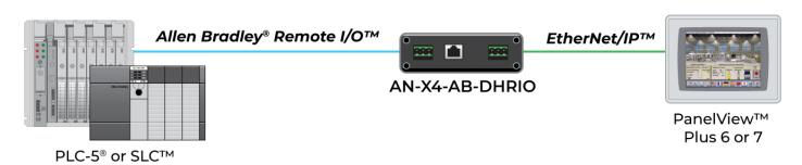
This operating mode allows legacy PanelViews to be upgraded to a PanelView Plus 6 or PanelView Plus 7 via EtherNet/IP.
