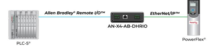
This operating mode supports upgrading legacy Allen Bradley drives on Remote I/O to new EtherNet/IP-enabled drives.
