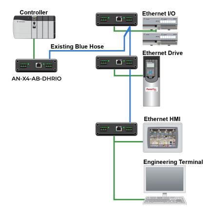
This operating mode allows the module to listen to all messages on an Ethernet network and use its "BridgeIP" mapping to forward the messages out of the DH+/BH port. The messages received on the DH+/BH port can be forwarded to the devices connected to its Ethernet port.
