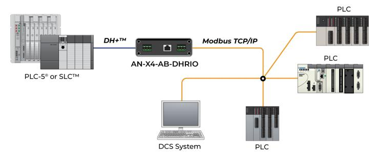
This operating mode allows Modbus TCP Clients to access the PLC data from stations on a Data Highway Plus Network.
