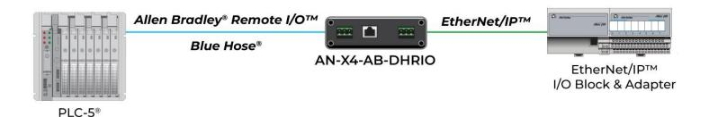
This operating mode allows PLC's on Remote I/O to connect to and control 1794-AENT EtherNet/IP Flex adapters.
