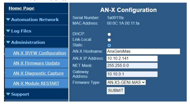
The serial number and MAC address of the AN-X being configured are shown.
