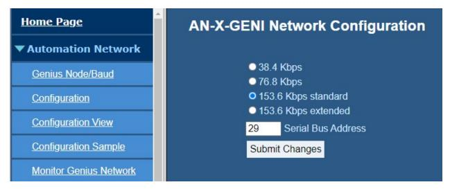
Check the desired baud rate from the four supported baud rates: 38.4Kbps, 76.8 Kbps, 153.6 KBPS standard or 153.6 Kbps extended. This setting MUST match the existing Genius network settings.
