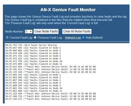
The web interface displays the faults in the Genius IO Fault Log area of the screen. To clear faults for a specific Genius block, select the serial bus address of the module from the *Station Number* list, then click the *Clear Station Faults* button.
