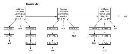
DI Pnts are generated for each command with an object type of 1.
