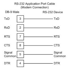
The *Use CTS Line* parameter for the port configuration should be set to **YES** for most modem applications.
