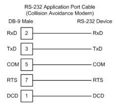
If collision avoidance is used in a point-to-point connection on the RS-232 interface, the following cable should be used.
