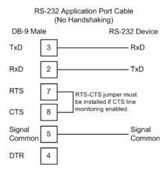
Note: If the port is configured with the *Use CTS* set to YES, then a jumper is required between the RTS and the CTS line on the module connection.
