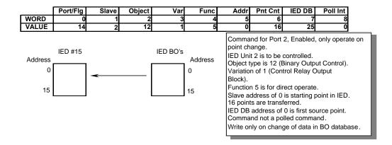
Note: CROB commands (object 12) exceeding a count of 16 are not recommended. Many IEDs only support one transport layer and a count > 16 may cause the IED device to not accept the new data value being written by the ProLinx module.
