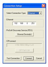
You can also use CIPconnect<sup>®</sup> to connect to the module through a 1756-ENBT card by choosing 1756-ENBT in the **Select Connection Type** list. Refer to Using CIPconnect<sup>®</sup> to Connect to the Module (page 44) for information on how to construct a CIP path.
