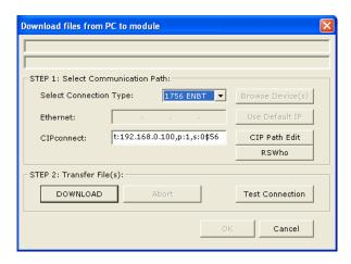
3 Click **RSWHO** to display modules on the network. The MVI56E-DNPNET module will automatically be identified on the network.
