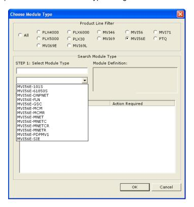
2 In the *Product Line Filter* area of the dialog box, select **MVI56E**. In the *Select Module Type* dropdown list, select **MVI56E-DNPNET**, and then click **OK** to save your settings and return to the *ProSoft Configuration Builder* window.
