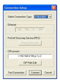
5 Configure the path as shown in the following illustration and click **Construct CIP**PATH to build the path in text format.
