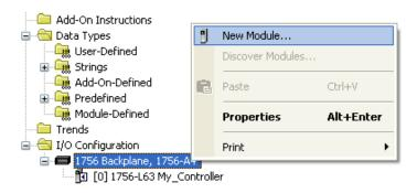
This action opens the **SELECT MODULE** dialog box. Enter *generic* in the text box and select the **GENERIC 1756 MODULE**. If you're using a controller revision of 15 or less, expand **OTHER** in the **SELECT MODULE** dialog box, and then select the **GENERIC 1756 MODULE**.
