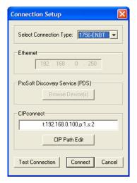
5 Configure the path as shown in the following illustration, and click **CONSTRUCT CIP**PATH to build the path in text format.
