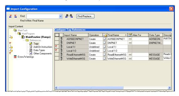
10 Associate the I/O connection variables to the correct module in the corresponding slot number. The default values are Local:1:I and Local:1:O and must be edited if the card is placed in a slot location other than slot 1 (Local:1:x means the card is located in slot 1). Since the second card is placed in slot 2, edit the FINAL NAME to Local:2:I and Local:2:O.
