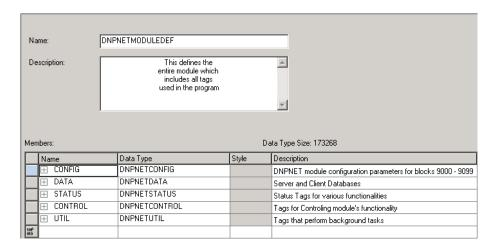
Click the [+] signs to expand the UDT structures and view lower-level UDTs. For example, when DATA is expanded, it contains four UDTs: DNPout, IEDin, DNPin, and IEDout. They can further be expanded with the [+] sign.
