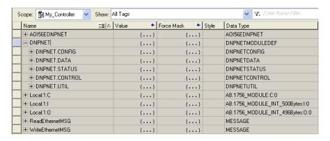
Some UDTs hold process or status data (*Module Data Objects*). This data can be monitored and manipulated by the application-specific ladder logic program. Other UDTs are used to store and organize the parameters needed for special functions and control features (*Special Data Objects*). These data types will be discussed in more detail in succeeding topics.
