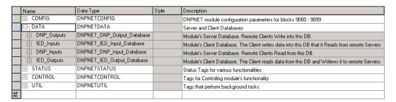
Notice these UDTs are the data types used to declare the DNPNET.DATA controller tag arrays.
