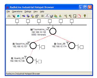
The Topology view shows a diagram of the network's wireless connections. Use this view to see whether all the radios are linked, and that you approve of the way the radios are linked. A radio that is not linked to a parent will show as a circle outlined by a flashing dashed red line. It may be near the bottom of the window, so scroll down to view all available radios. To change how radios link to the network, see Parent Link settings.
