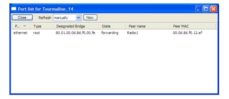
The port table is a list of all the active ports on the radio. This list shows the same information as the Port status (page 44) list in the Radio Configuration / Diagnostic Utility. Each radio can have up to 34 active ports—one Ethernet cable, one parent RF link, and up to 32 child RF links.
