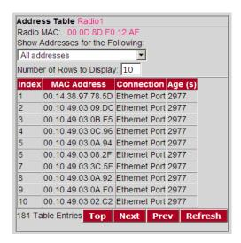
The Address Table shows the port through which each MAC address is connected, along with the age in seconds since the radio last saw a packet from this MAC address.
