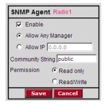
SNMP is a network management protocol that is often used with TCP/IP and Ethernet. As an alternative to using the Radio Configuration / Diagnostic Utility, you can change radio settings and view diagnostics in an SNMP manager application, if necessary.
