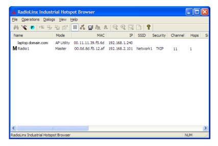
The window lists all the radios your computer can access. The MAC ID number is essentially the serial number of the radio; this number is also printed on the side of the radio. If a radio listing does not appear in the window, select Scan from the File menu.
