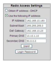
If a DHCP (Dynamic Host Control Protocol) server is configured on your local area network, the DHCP server can assign IP addresses automatically. If you prefer to assign a Static (Fixed) IP address, select "Use the following IP address", and then enter the IP Address, Subnet Mask and Default Gateway in the Radio Access Settings area of the IH Radio web configuration form.
