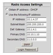
In order to configure or diagnose a radio using its built-in Web server or SNMP agent, both your computer and the radio must have IP addresses, and these IP addresses must be on the same subnetwork. An IP address is only needed so you can configure the radio and view its diagnostic settings. Otherwise, the address is unnecessary.
