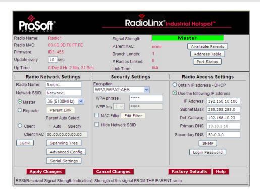
To configure a Master radio, make the following changes to the web configuration form:
