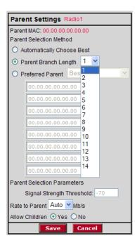
With **Parent Branch Length**, the IH will choose its parent strictly by the number of repeaters between it and the Master radio. If Branch Length of 1 is chosen, the IH will link only to the Master radio. If Branch Length of 2 is chosen, the IH will link only to an IH that is linked to the Master radio, and so on.
