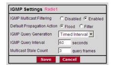
RLXIB-IHG radios support IGMP v1 and v2. The default operation of the RLXIB-IHG radios is to have IGMP functionality enabled, although the user can disable IGMP entirely. Additionally, the user can specify settings associated with IGMP filtering and snooping. Unknown multicast addresses can be sent to all ports (flood) or to none (filtered) by changing the IGMP Multicast Filtering option. The user can specify whether the radio will generate IGMP queries, and configure the query interval time.
