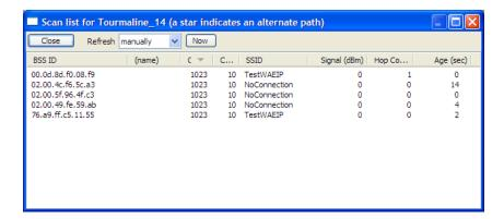
The scan list is a list of all the radios that this particular radio "hears" on this channel (via beacons) even if it is not linked to it (different SSID or encryption). This list shows the same information as the Available Parents list in the Radio Configuration / Diagnostic Utility.
