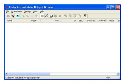
The window lists all the radios your computer can access. The MAC ID number is essentially the serial number of the radio; this number is also printed on the side of the radio. If a radio listing does not appear in the window, select Scan from the File menu. If you still do not see a radio listing, see Troubleshooting.
