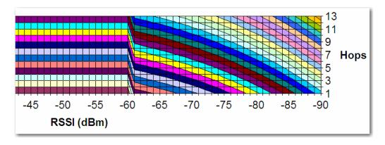
Once per second the RLXIB-IHG radio evaluates the link it has to its parent to determine if this link is the best parent to use. A cost is calculated for each entry and can be seen in the column labeled "Cost" in the preceding table. The cost calculation is based not only on the strongest signal, but on several other factors to provide optimum network communication.
