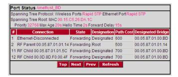
When you click the Port Status button, you can see information about all the active ports on the radio. Above the table, you can see information about the current Spanning Tree (page 54), including the MAC address of the "root" device, and the timing parameters that are set for the current Spanning Tree. Each radio can have up to 34 active ports—one Ethernet cable, one parent RF link, and up to 32 child RF links.
