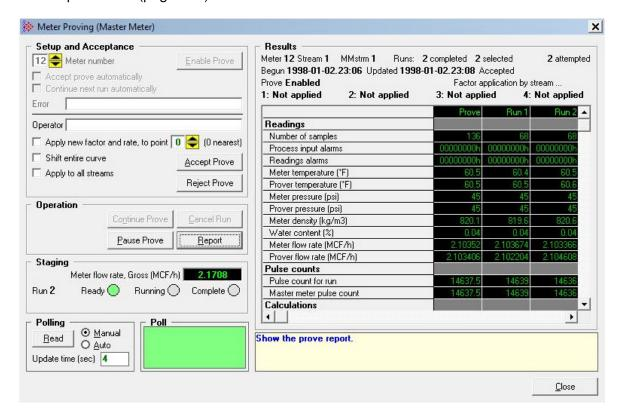
The *Meter Proving* window above shows the system during a prove using a Master Meter. Notice the differences in the example of the information that is available before and after connecting to the module.
