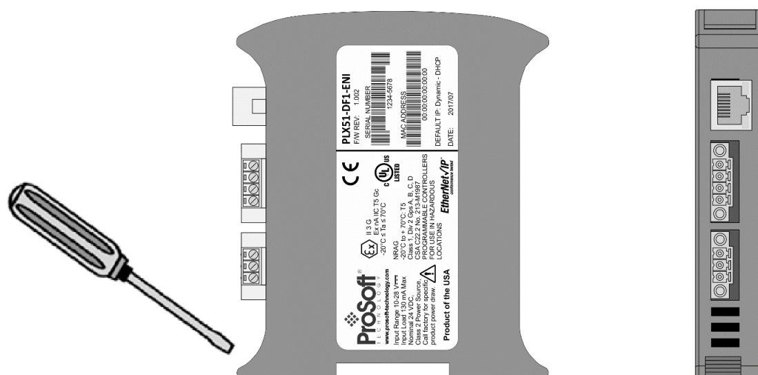
Figure 2.4 - DIN rail mounting
