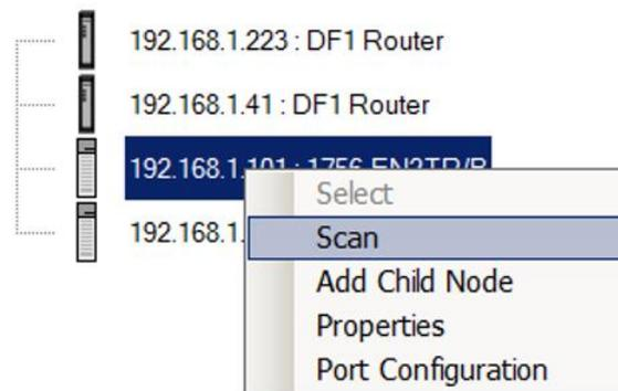
Figure 3.21. - Scanning node in the Target Browser
