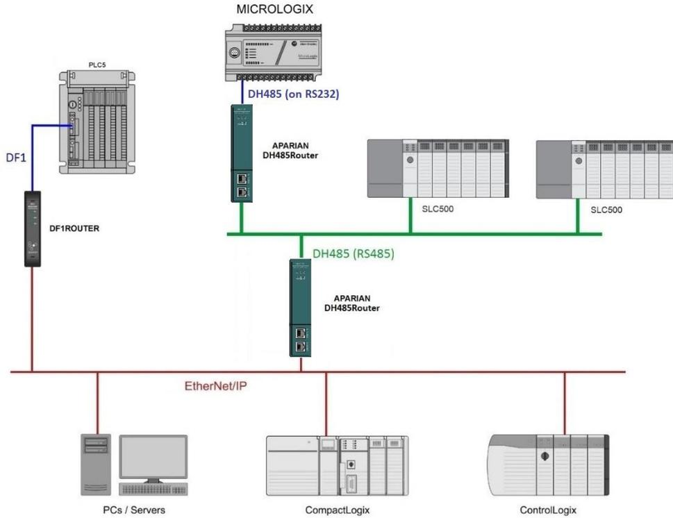
Figure 1.6. - Example of a new network setup
