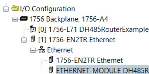
Figure 3.51 - RSLogix 5000 I/O module tree
