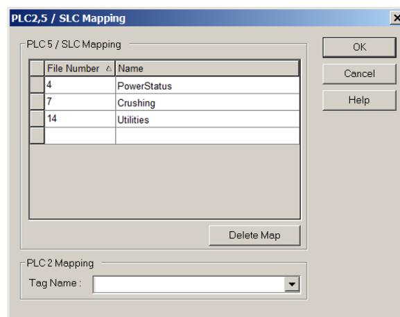
Figure 3.31 - Example of Mapping PLC/SLC Messages in RSLogix 5000
