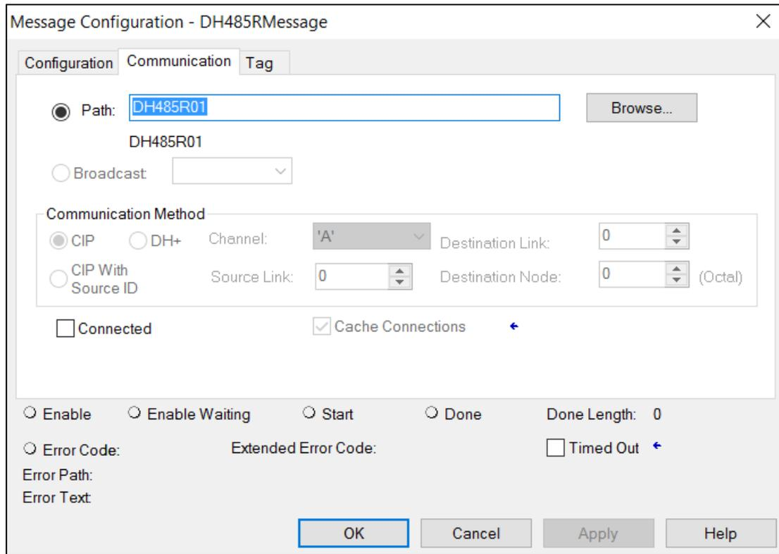
Figure 4.4. - Message Configuration - Communication
