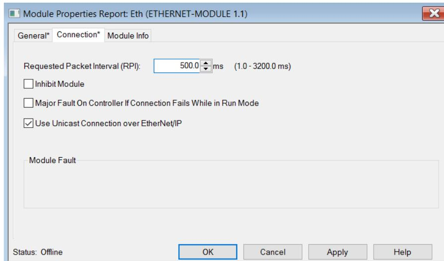
Figure 3.50 - Connection module properties in RSLogix 5000
