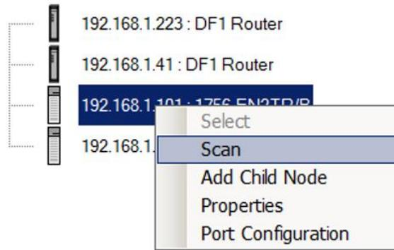
Figure 3.33 - Scanning node in the Target Browser
