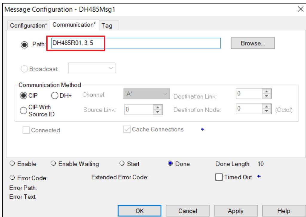
Figure 4.8. – Logix SLC Read/Write Communication Path
