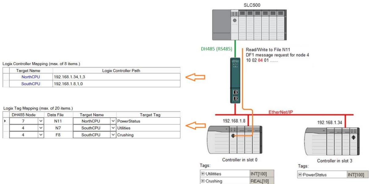
Figure 3.37 - Reactive Tag mode configuration in Slate
