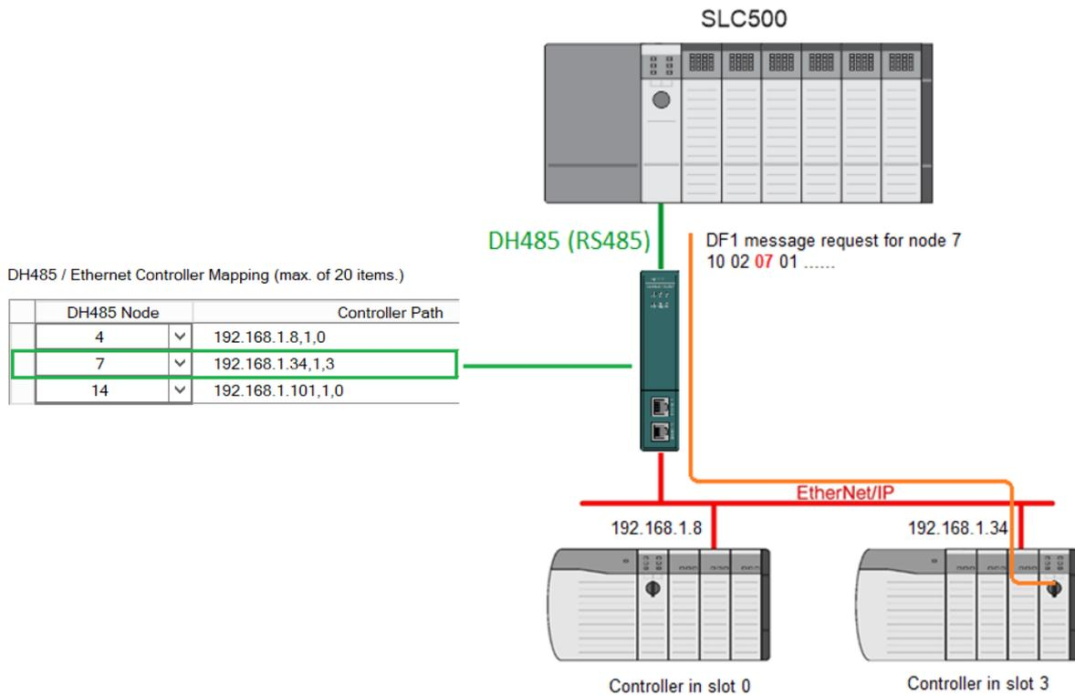
Figure 3.30 – Example 2 – Transparent routing map – node 7
