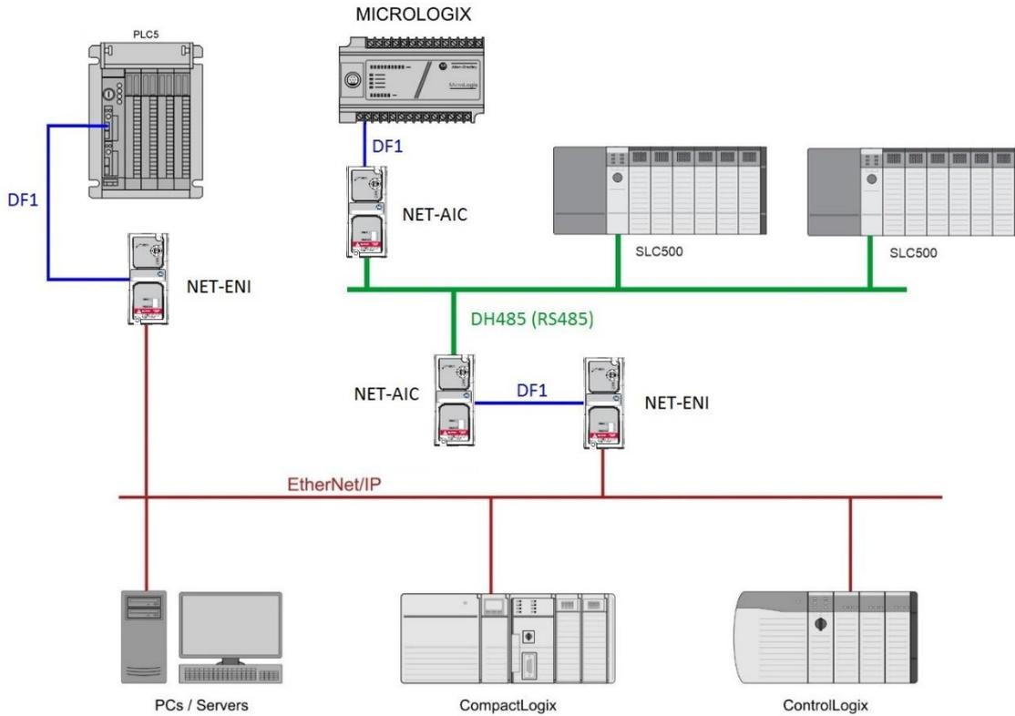
Figure 1.5. - Example of an old network setup
