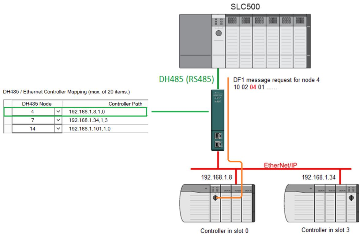
Figure 3.29 – Example 1 - Transparent routing map – node 4
