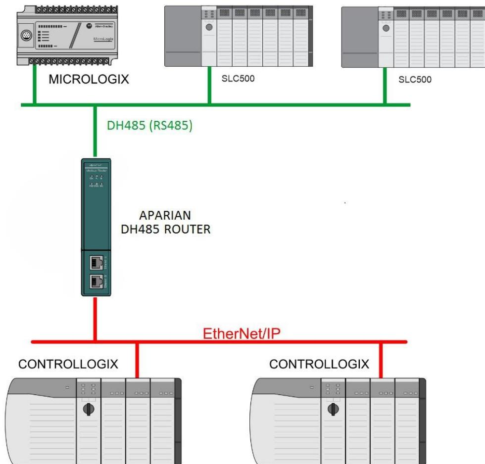
Figure 1.1. - Example of a typical network setup
