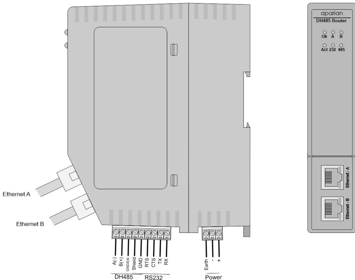
Figure 2.1. - DH485 Router/B side and front view
