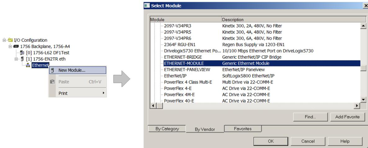
Figure 3.48 - Add a Generic Ethernet Module in RSLogix 5000
