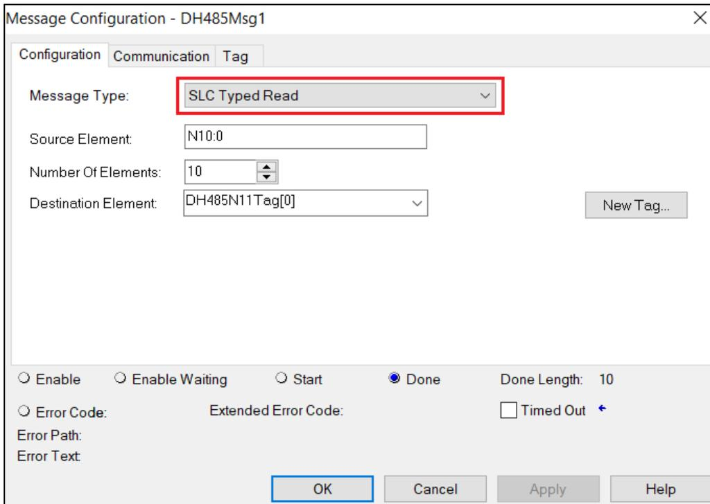
Figure 4.7. – Logix SLC Read/Write Message Type
