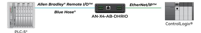
This operating mode allows PLC's on Remote I/O to share data with a newer ControlLogix or CompactLogix PAC's. This mode also allows a ControlLogix processor to monitor Block Transfer and I/O data on an active Remote I/O network without occupying a drop.
