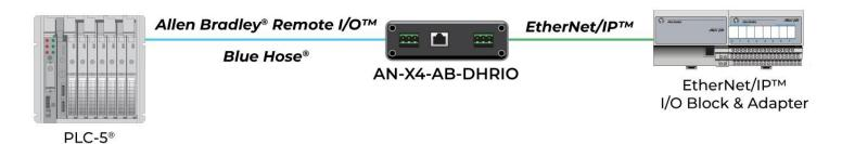
This operating mode allows PLC's on Remote I/O to connect to and control 1794-AENT EtherNet/IP Flex adapters.
