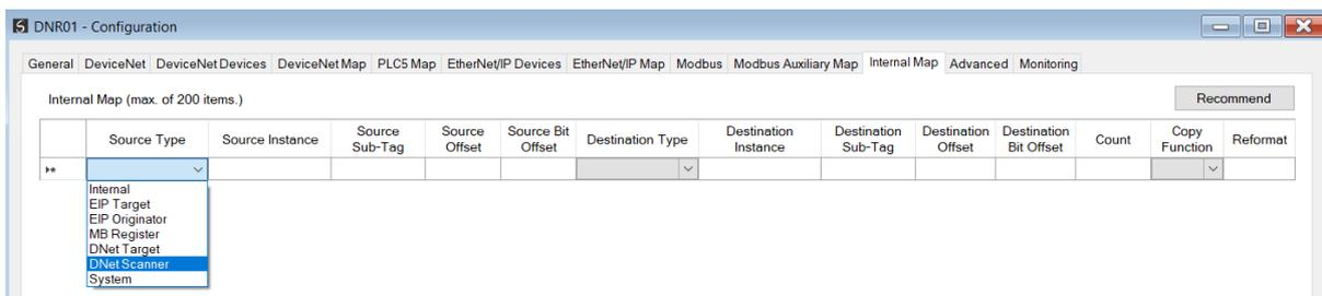
Figure 3.136 – IDS Copy – DeviceNet Scanner Source Type
