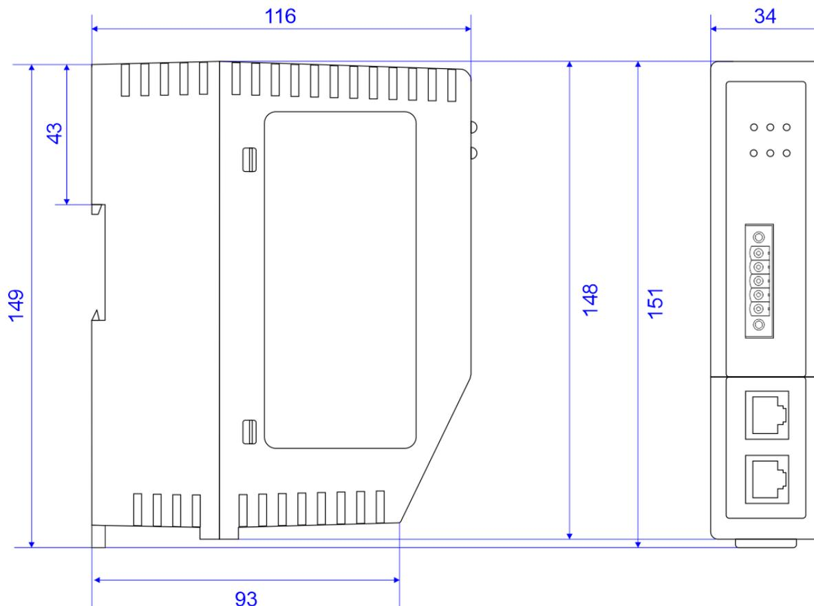
Figure 7.1 – DeviceNet Router/B enclosure dimensions
