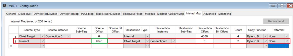
Figure 5.25 – Explicit Messaging – Internal Mapping from IDS to DeviceNet
