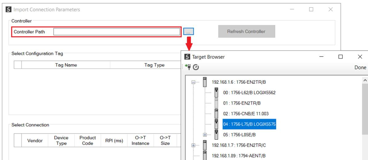
Figure 3.110 – Import Connection Parameters – Controller Path
