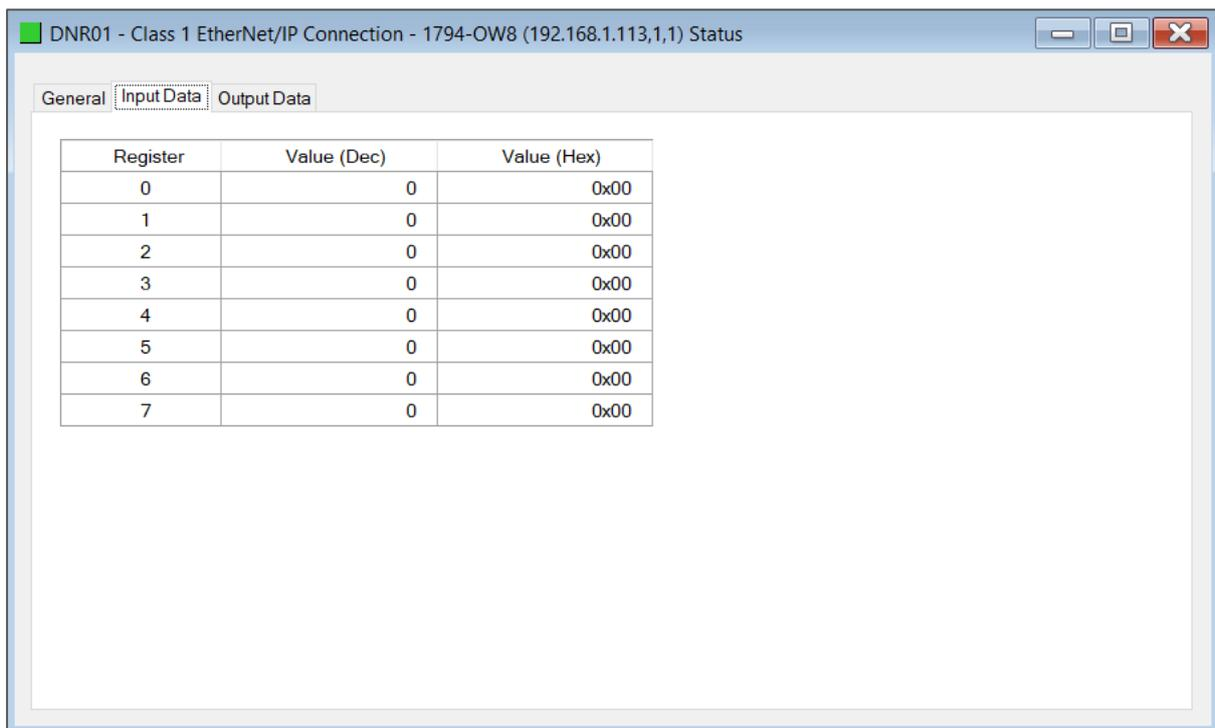
Figure 6.19 – EtherNet/IP Device Status – Input Data
