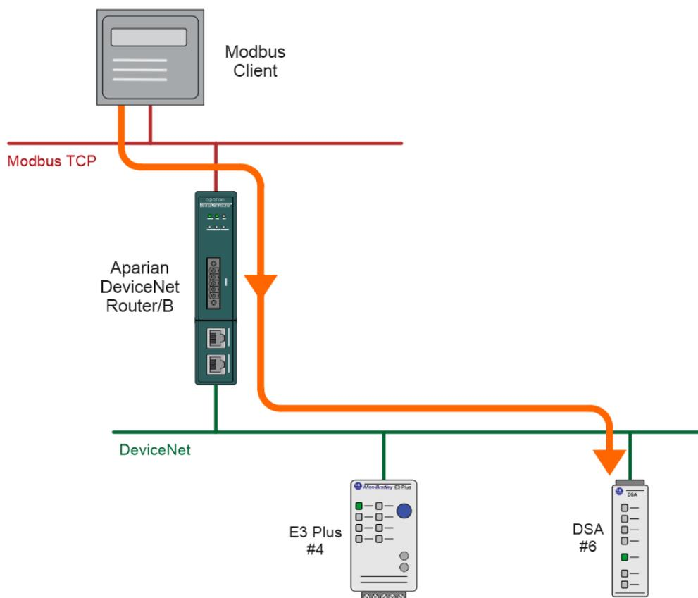
Figure 5.29 – Modbus TCP Client to DeviceNet IO operation
