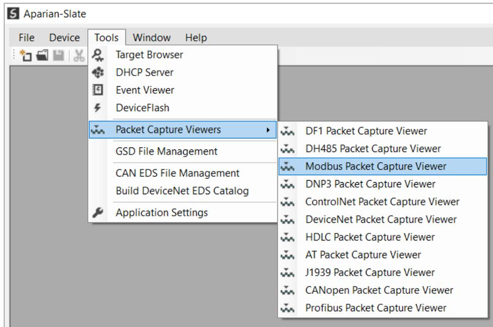
Figure 6.35 - Selecting the Modbus Packet Capture Viewer
