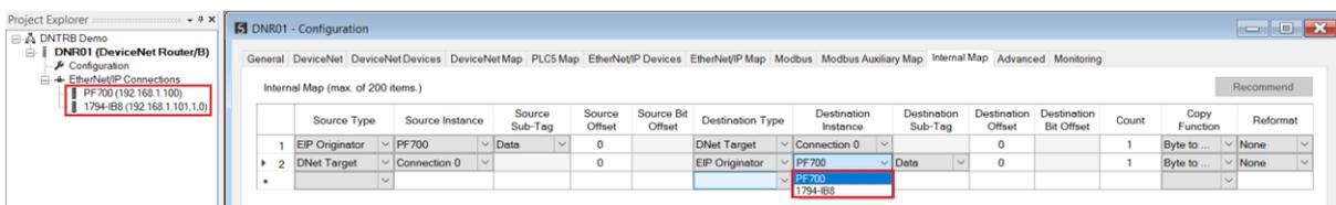
Figure 3.144 – IDS Copy – EtherNet/IP Originator Destination Instance
