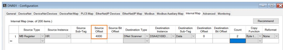
Figure 5.30 – Internal Mapping from Modbus Register to DeviceNet IO
