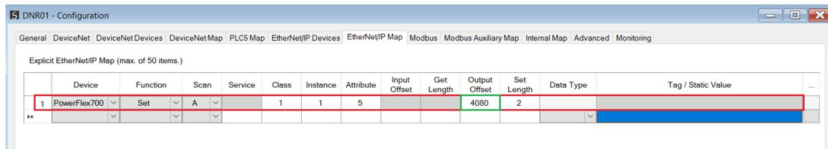
Figure 5.23 – Explicit Messaging – Set Function from IDS to EtherNet/IP device
