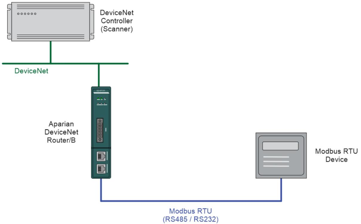
Figure 1.7. – Modbus RTU Device (Client or Server) operating as a DeviceNet Device
