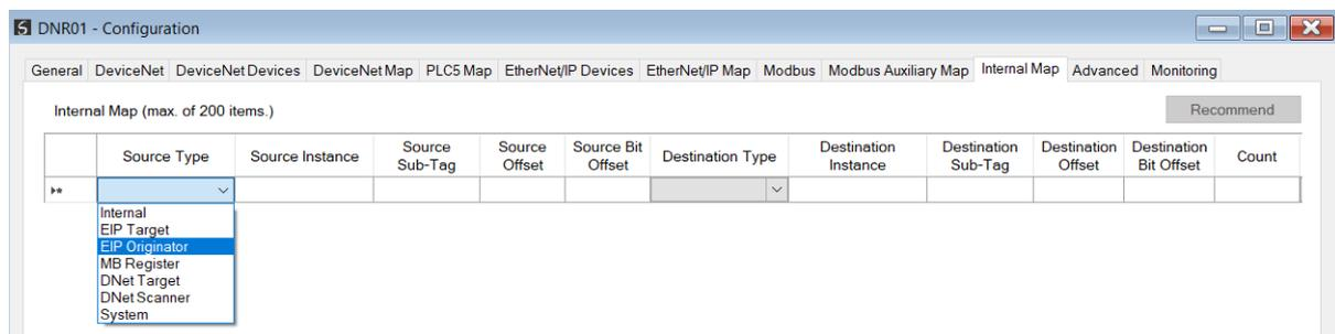
Figure 3.122 – IDS Copy – EtherNet/IP Originator Source Type
