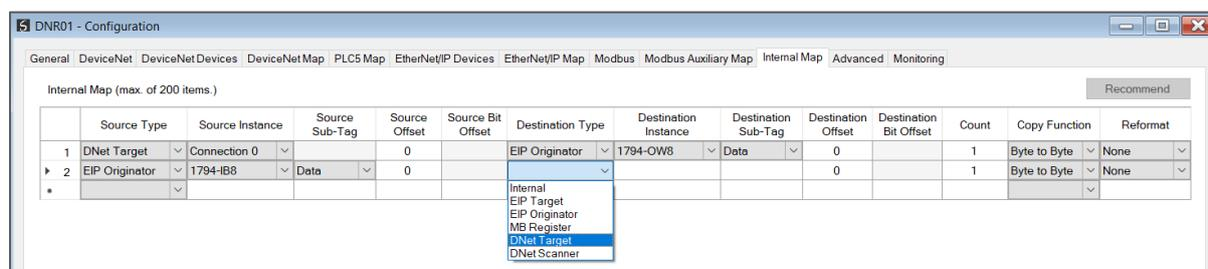
Figure 3.147 – IDS Copy – DeviceNet Target Destination Type
