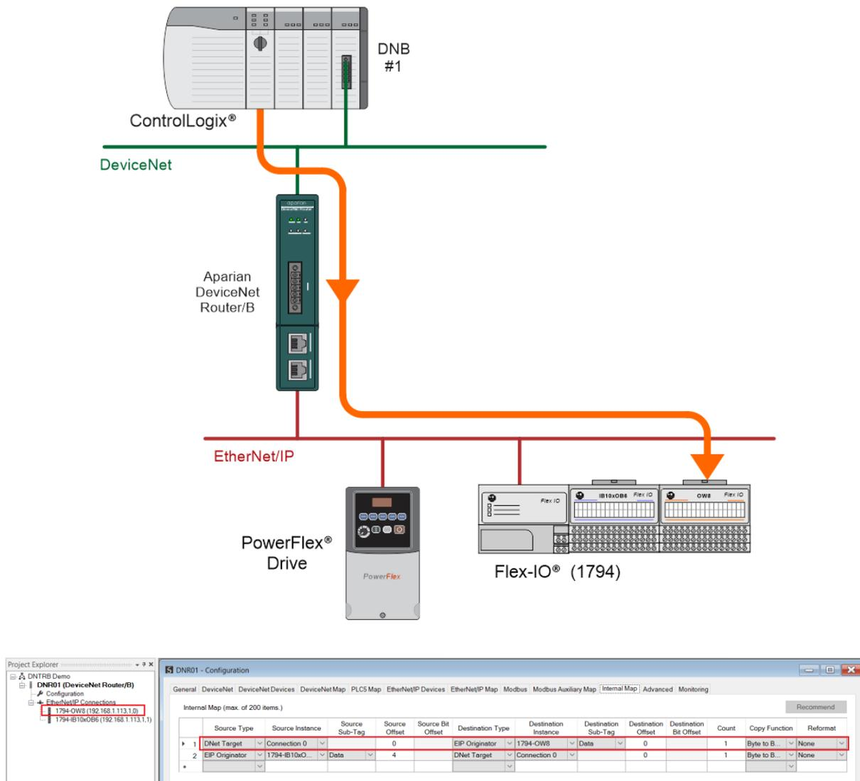
Figure 5.19 – Internal Mapping from DeviceNet to EtherNet/IP Originator
