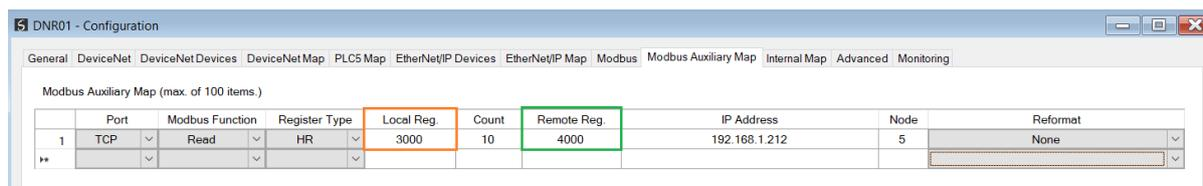
Figure 5.27 – Modbus Client Aux Mapping
