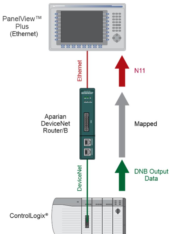
Figure 5.32 – PanelView reading Logix data over Cyclic DeviceNet
