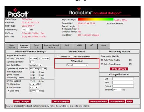
**Note:** The default *RF Medium* setting is **Normal**. If set to **Discontinuous** mode it must be set on both AP and Client. In the Client, setting to Discontinuous mode will also automatically result in the following configuration changes:
