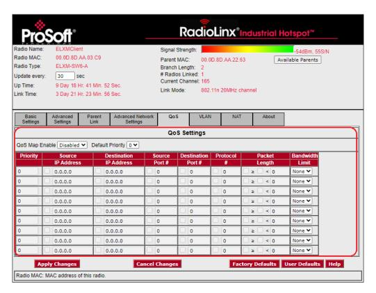
The ELXM-SW6 prioritizes frames using QoS for packets received already marked with a priority value. The QOS Settings tab allows you to set the default priority for frames that the ELXM-SW6 receives without any priority markings. In addition, priority values can be mapped to packets received without priority markings according to a set of matching criteria.
