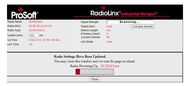
7 After successfully rebooting, the ELXM-SW6 appears as an Ethernet Bridge radio in the IH Browser window:
