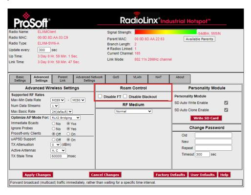
In roaming applications, a mobile platform equipped with the ELXM-SW6 roams from one AP radio's coverage area to another radio's coverage area. By default, a Client radio roams automatically by calculating the cost for each roam candidate based only on RSSI and hop count. A lower cost determines when a better Parent radio candidate is present.
