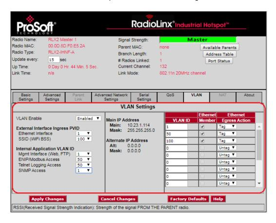
ELXM-SW6's support port based VLANs. Each ELXM-SW6 can be considered to have 3 different ports or interfaces; the Ethernet interface, the local applications stack of the ELXM-SW6 itself, and the 802.11 BSS created by each AP.
