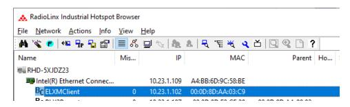
8 If there is an AP with the correct credentials nearby, the Bridging Client should wirelessly connect. In this mode, multiple Ethernet devices can connect with any 3rd-party access points (802.11 a/b/g/n/ac/ax).
