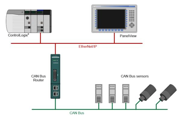
Figure 1 – Example of connecting CAN Bus sensors to a Logix Controller
