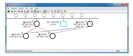
**Note:** You can also display a detailed list of each of the alternate Parent radios by right-clicking a radio and choosing **SCAN LIST**. This list shows the RLX2/ELXM series radios in the same network and all 802.11 Access Points on other networks. For more information, see section 9.3 Viewing the Scan List in the IH Browser.
