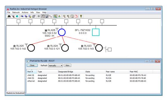
The port table is a list of all the active ports on the radio. Each RLX2/ELXM series radio has up to 252 active ports: one Ethernet wired port, one parent radio frequency link, and up to 250 child radio frequency links.
