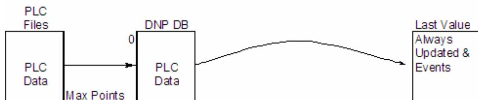
All data for these data types is derived from the processor and is passed to the module over the backplane. The module will constantly monitor for changes in this data and generate event messages when point values change. For binary input points, events will be generated on any state change. For analog input points, events will be generated for points that have a current value outside of the user-set deadband based on the last value used for an event.
