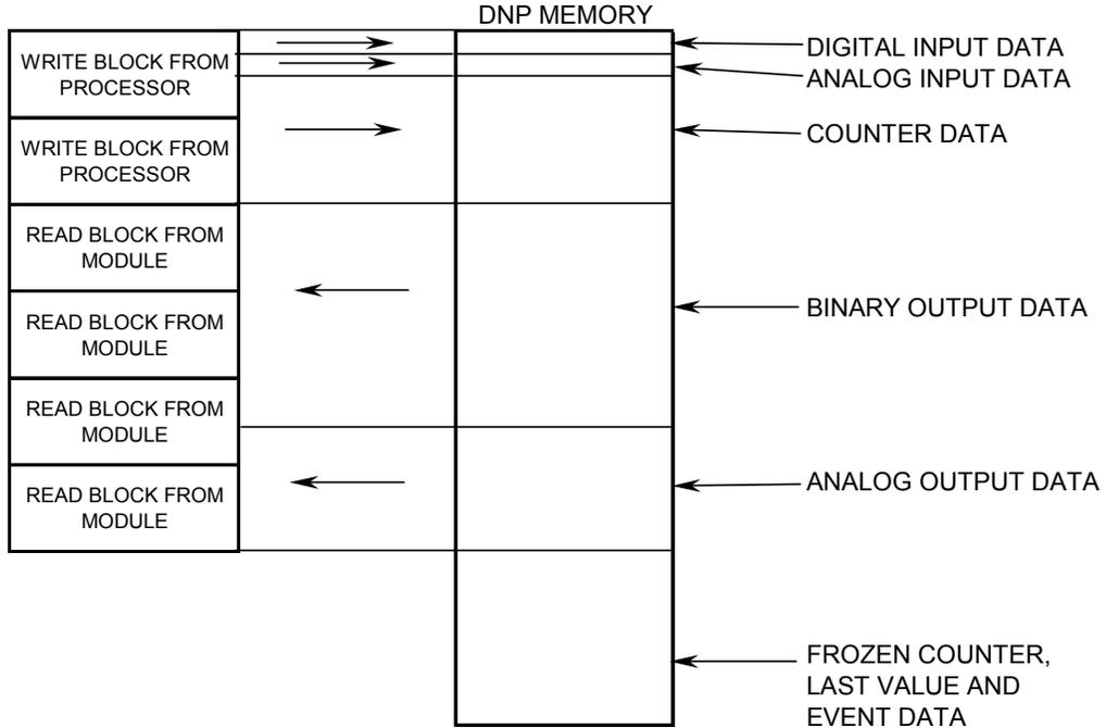
It is important to understand the relationship of the block identifications and the data in the module.
