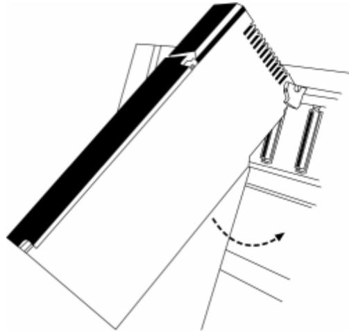
**CaUTION:** The PTQ module is hot-swappable, meaning that you can install and remove it while the rack is powered up. You should not assume that this is the case for all types of modules unless the user manual for the product explicitly states that the module is hot-swappable. Failure to observe this precaution could result in damage to the module and any equipment connected to it.
