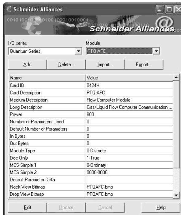
Now you can close the Schneider alliances application and run the Proworx 32 software. At the Traffic Cop section, select the PTQ module to be inserted at the slot:
