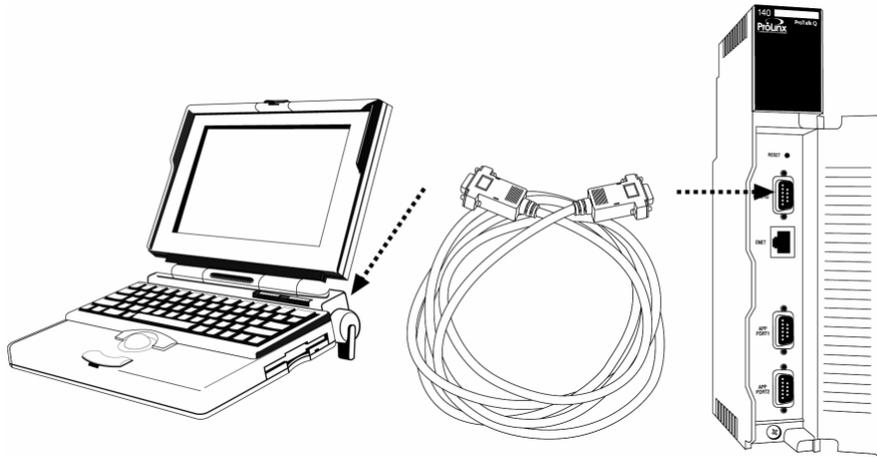
To connect to the module's Configuration/Debug serial port:
