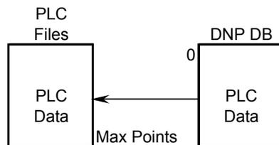
Output data is sourced from the controlling master station and passed to the processor over backplane from the module. These data are used in the ladder logic to control operations and I/O in the processor.
