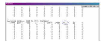
The data shown represents clock values originating from the 6201-WA-ASCII module. The values are stored in 5 registers beginning with register 3000. The clock values are being passed wirelessly to the 6201-WA-DFNT. The 6201-WA-DFNT module is taking this data and passing it back to the 6201-WA-ASCII module and placing it into 5 registers beginning at register 3005.
