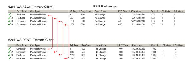
Both the ASCII and the DFNT have corresponding Produce and Consume commands. The following diagram illustrates the sample application:
