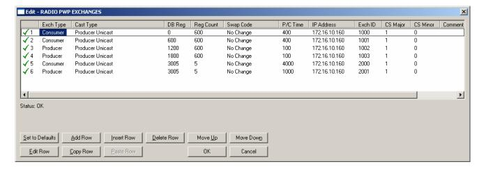
This is the area where you set up data exchange between the ASCII and the DFNT modules. Communication is accomplished using Producer and Consumer commands. Using these commands, you specify the IP address of the receiving (Consumer) and sending (Producer) module as well as the database locations to produce data and receive data.
