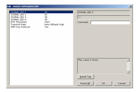
The default Signal LED 1 through 4 parameter values are fixed and cannot be modified. If you need to change the values for the remaining parameters in this dialog box, make sure to save your changes before moving on to the next step. As you select each parameter, the help text area in the lower right area of the dialog box displays information to help you make your selections.
