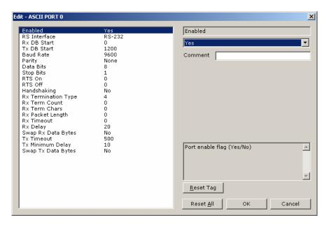
The remaining parameters are set to ensure that the ASCII module can communicate with the PLC. Refer to the ASCII Driver Manual located on the ProLinx solutions CD for detailed information on each of these parameters.
