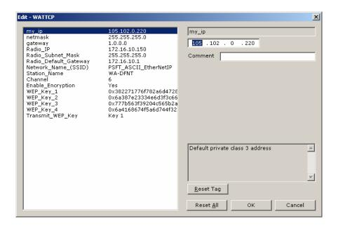
Every EtherNet/IP module is set up with the defaults shown in the example. You may have to modify values such as the Radio Default Gateway, the Network Name (SSID), and the Station Name to suit the needs of your network. The Station Name may be modified when using more than one EtherNet/IP module.
