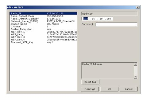
Every ASCII module is set up with the defaults shown in the example. You may have to modify values such as the Radio Default Gateway, the Network Name (SSID), and the Station Name to suit the needs of your network. The Station Name may be modified when using more than one ASCII module.
