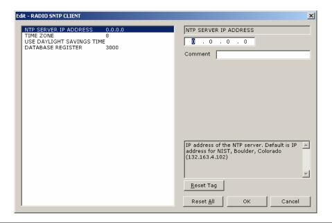
This section is used to synchronize the time using a centralized atomic clock. This feature is only usable if your modules are communicating through an access point such as a RadioLinx Industrial Hotspot. The values in this window should be left with the default values. As you select each parameter, the help window on the screen displays information to help you make your selections. The PWP Driver Manual located on the ProLinx Solutions CD describes each parameter in detail.
