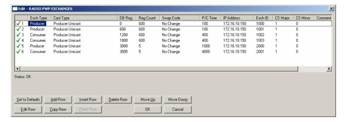
This is the area where you set up data exchange between the modules. Communication is accomplished using Producer and Consumer commands. Using these commands, you specify the IP address of the receiving (Consumer) and sending (Producer) module as well as the database locations to produce data and receive data.
