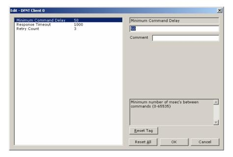
The remaining parameters are set to ensure that the DFNT module can communicate with the PLC. Refer to the DFNT Driver Manual located on the ProLinx solutions CD for detailed information on each of these parameters.
