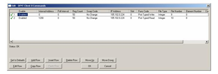
**Note:** For command lines 1 and 2 to function properly with the ControlLogix processor, the menu item "Logic/Map PLC/SLC Messages..." in the RSLogix 5000 application, must have the "File Number" field in the "PLC 2, 3, 5/SLC Mapping" dialog box linked/associated with a user specified "Tag Name" Field Tag.
