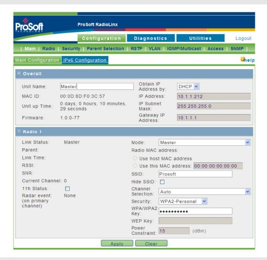
**Important:** In order to connect to a RLXIB-IH2N-W radio from a web browser or SNMP agent, both your computer and the radio must have IP addresses, and these IP addresses must be on the same subnet.
