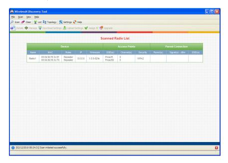
The window lists all the radios your computer can access. The MAC ID number is essentially the serial number of the radio; this number is also printed on the side of the radio. If a radio listing does not appear in the window, click the **SCAN** button on the toolbar. If you still do not see a radio listing, refer to Diagnostics and Troubleshooting (page 41) in the RLXIB-IH2N-W User Manual.
