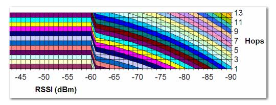
Once per second, the RLXIB-IH2N-W radio evaluates the link it has to its parent to determine if this link is the best parent to use. A cost is calculated for each entry and can be seen in the column labeled "Cost" in the preceding table. The cost calculation is based not only on the strongest signal, but on several other factors to provide optimum network communication. There is built in hysteresis to prevent frequent link fluctuations.
