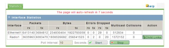
**Note**: Each Radio's configuration is unique. If the hardware supports more than one physical radio, and more than one Ethernet port, the traffic statistics are cumulative for each pair.
