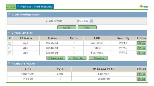
A given radio can have multiple virtual APs (VAPs) configured on it, and these virtual APs can be active concurrently. There is a general mode AP that is the default link for parent and child connections. This general mode AP is VLAN-aware, in that there is filtering for VLAN tags enabled along this link.
