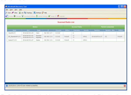
The Radio List has a table of detected radios in the network. This table allows you to identify radios by role, MAC address and device name. If a particular radio has parents or children in the network, they are identified by MAC address, SSID and security for that wireless link. Clicking on the column heading lets you to sort the list (in ascending or descending order) based on the selected field.
