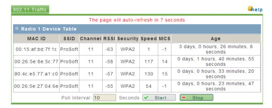
Depending on the radio's Radio's configuration, this list may include 802.11 devices that are members of other SSIDs.
