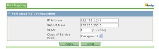
These mappings apply to the traffic originating from VLAN unaware devices, and have higher preference over the PVID setting on the link.
