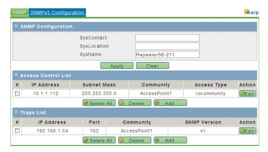
The RLXIB-IH2N-W SNMP agent supports the SNMPv2c and SNMPv3 protocol versions, and can send traps to a specified community.
