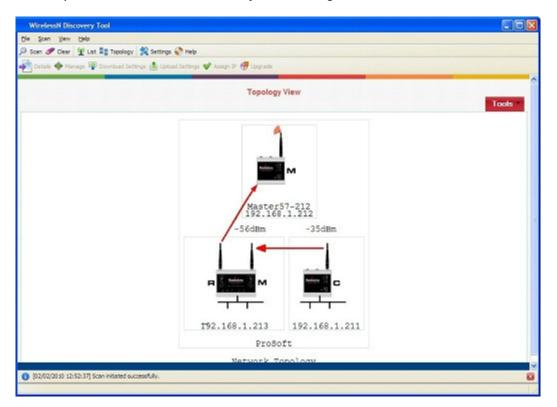
Each radio icon has a letter icon that corresponds to the role - M for Masters, R for Repeaters, and C for Clients. In the case of a device with two radios (i.e. two WLAN cards) each having a different role, a letter is shown on the left and right sides of the image in the topology view, indicating the function of each WLAN card. For example, the radio in the following illustration has one card configured as a Master, and the other card configured as a Repeater.
