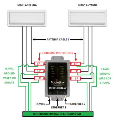
Ground wires or straps must be tied from each active lightning protector to a secured earth ground.
