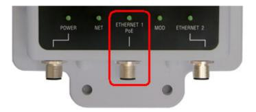
From left to right: Power, Ethernet 1, and Ethernet 2 Use the Ethernet cable to configure the radio for the first time. RLXIB-IH2N-WC has the connection shown below and differs from the RLXIB-IH2N-W.
