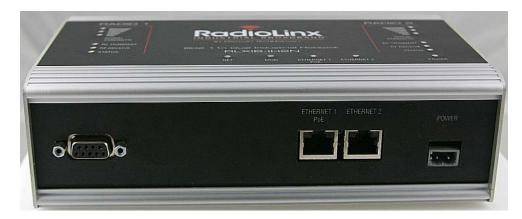
From left to right: Serial, Ethernet 1, Ethernet 2, and Power Use the Ethernet cable to configure the radio for the first time.
