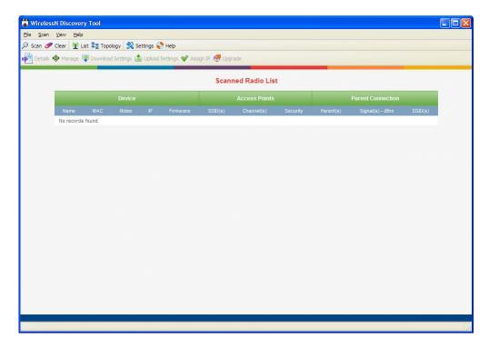
The window lists all the radios your computer can access. The MAC ID number is essentially the serial number of the radio; this number is also printed on the side of the radio. If a radio listing does not appear in the window, click the **SCAN** button. If you still do not see a radio listing, see Troubleshooting in the RLXIB-IH2N User Manual.
