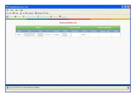
The window lists all the radios your computer can access. The MAC ID number is essentially the serial number of the radio; this number is also printed on the side of the radio. If a radio listing does not appear in the window, click the **SCAN** button on the toolbar. If you still do not see a radio listing, refer to Diagnostics and Troubleshooting in the RLXIB-IH2N User Manual.
