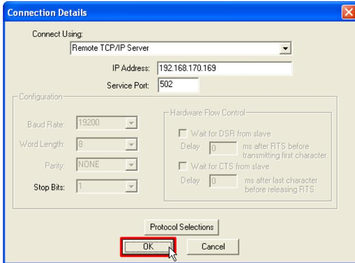
Click on ok to start the exchanges between the Client TCP and the Modbus slave.
