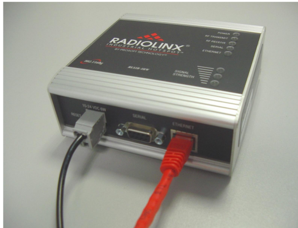
From left to right: Power connector, serial port and Ethernet port.
