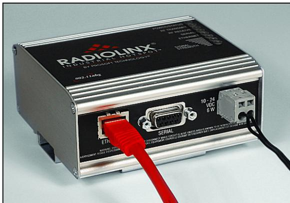
From left to right: Ethernet port, serial port and power connectors.
