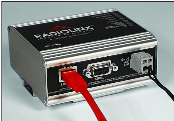
From left to right: Ethernet port, serial port and power connector.
