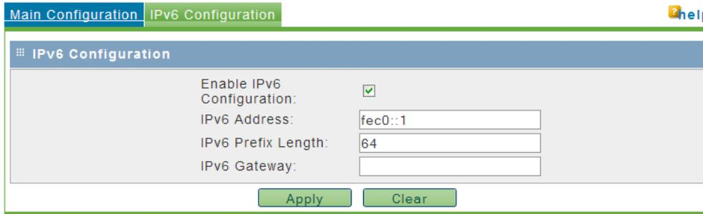
Enter the following parameters to configure the static IPv6 networking:
