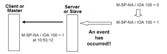
The following illustration shows the event communication between the Master and the gateway during unbalanced mode:
