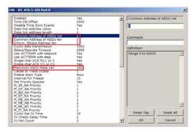
The Common Address of ASDU is the station address. The gateway allows the addressing of only the whole station (some devices allows different Common Addresses to identify particular station sectors). You should configure the Common ASDU Address with the following parameter:
