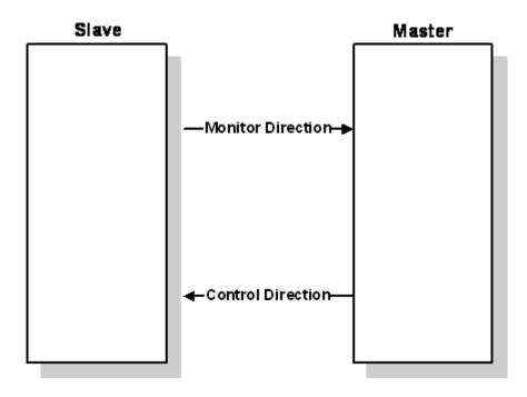
The points that are typically transferred from the slave to the Master are also known as Monitor Points (or Monitor Information Objects). The points that are typically transferred from the Master to the slave are also known as Control Points (or Command Information Objects).
