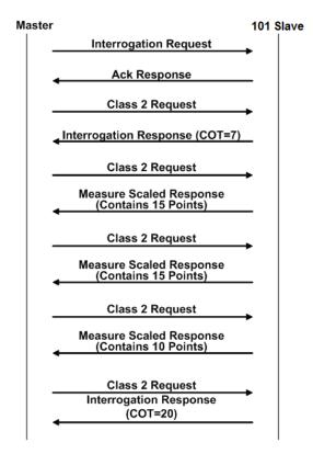
As shown in the previous diagram, the gateway sends out three (3) messages (15 points, 15 points, and 10 points) instead of sending the whole 40 points in one single message.
