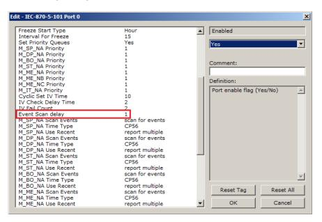
If this parameter is set to 0, the gateway will not generate events for any points. A non-zero value will configure how frequently the gateway will scan for events in the database.
