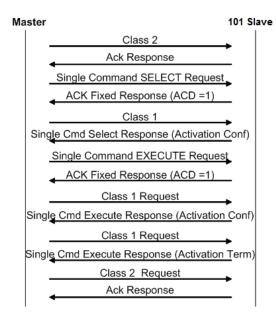
Refer to the following parameter to configure the select/operate timeout period. After the gateway receives the SELECT operation it will wait for this period of time for the EXECUTE operation. If the gateway does not receive an EXECUTE operation within this period of time it will require another SELECT operation before the EXECUTE operation.
