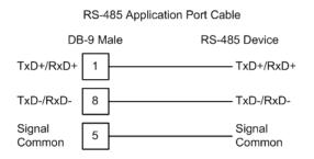
**Note:** Terminating resistors are generally not required on the RS-485 network, unless you are experiencing communication problems that can be attributed to signal echoes or reflections. In these cases, installing a 120-ohm terminating resistor between pins 1 and 8 on the gateway connector end of the RS-485 line may improve communication quality.
