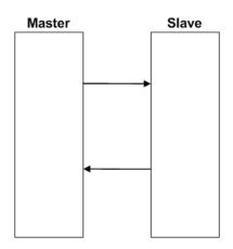
The gateway works as an IEC-60870-5-101 slave. It can send monitor data, receive commands or generate events to the Master unit, as explained in the following topics.
