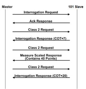
This example shows that the gateway sends all 40 measured scaled points in one single message, if the message is not greater than 252 bytes. However, some Master devices may not support messages containing this number of bytes. If the Master for a given application supports only 100 bytes, the following communication procedure would occur:
