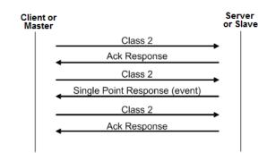
The gateway can queue up to 99 events per data type. When the queue is full, the oldest event will be deleted each time a new event is added to the queue. You must configure the Master to poll the event queue frequently enough to avoid losing events.
