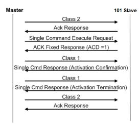
Some of the command points may be configured to be selected before executed. The following illustration shows a typical command communication between the Master and gateway operation with a SELECT operation.
