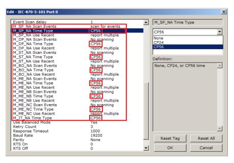
The Master should periodically send a Time Synchronization command to the gateway driver to synchronize its date and time information. This is a very important step in order to make sure that the Master and the slave are both using the same time information.
