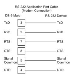
The "Use CTS Line" parameter for the port configuration should be set to 'Y' for most modem applications.
