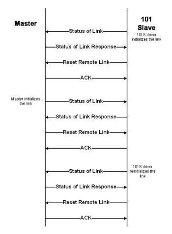
After the initialization procedure is completed, the Master and the 101S start communicating. During communication, if the Master fails to respond to a message from the gateway, the gateway will retry for a configured number of times. If the Master still fails to respond, the gateway will attempt to initialize the line again.
