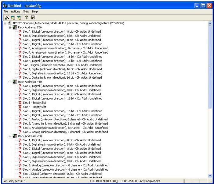
The IpcMasCfg tool will prompt the user for the RSLinx path to the QTS IPC-620 module and store this path for future communications with the scanner module (see status bar in diagram, above).
