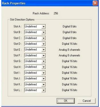
7. For each slot in the 'Rack Properties' dialog, set the slot direction (input or output) to match the physical card file configuration. Click the 'OK' button when all slots have been configured.
