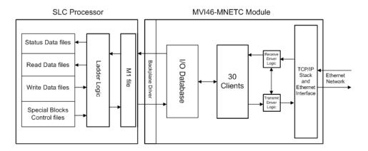
All data transferred between the module and the processor over the backplane is through the M1 file. Ladder logic in the SLC must interface the input and output image data with data defined in the SLC data files. All data used by the module is stored in its internal database. This database is defined as a virtual Modbus data table with addresses from 0 (40001 Modbus) to 4999 (45000 Modbus). The following illustration shows the layout of the database:
