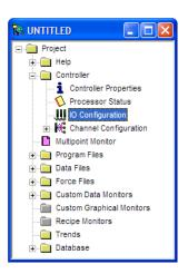
This action opens the I/O *Configuration* dialog box. Select an empty slot in the left pane, and then scroll to the bottom of the right pane.
