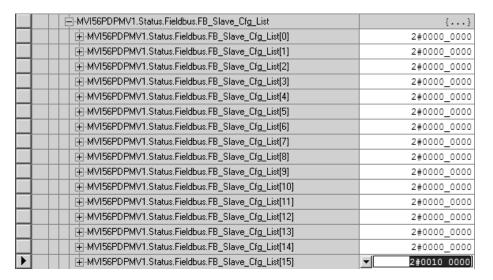
**Note:** For the FLEX sample program, you must toggle the command bit **MVI56PDPMV1.Command.GetStatus** in order to update the status data. For the LEGACY sample program the status data is updated automatically.
