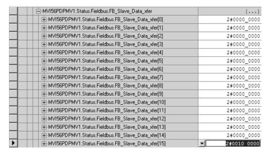
**Tip**: You can add ladder logic to perform an action based on the values of these tags, for example to determine if a slave is misconfigured.
