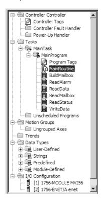
**9** Copy and paste each of the user-defined types from the sample ladder logic into your existing application.
