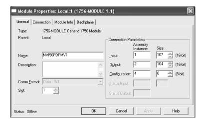
For this scenario, each backplane block reserves a maximum of 99 words for PROFIBUS I/O data. The configured PROFIBUS I/O size (100 words) will not fit into one block, so two backplane input blocks and two backplane output blocks will be required to transfer the entire PROFIBUS I/O data.
