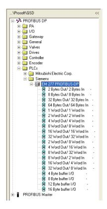
5 Drag the input and output parameters to the Slot Location Grid (Subscriber List) below the Bus Configuration window. This view displays the slot number, configuration data, and starting input and output addresses. The MVI56-PDPMV1 Master uses this information to identify and communicate with individual slaves on the network.
