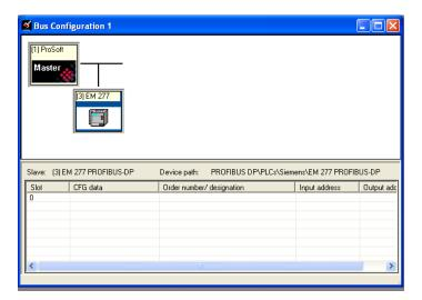
4 In the tree view, click the plus sign [+] to expand the slave device you added. This action opens a list of device configuration values. The following illustration shows the possible input/output configuration values for a Siemens EM 277 PLC Slave. The selections available for other devices will be different, so you should review the specifications for the product you are installing in order to determine the correct values to use.
