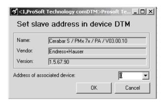
**Note**: You must use the same PROFIBUS device address that you used when setting up the device.
