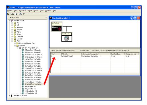
For each new slave added to the PROFIBUS network, PCB automatically converts the input/output byte addresses to word input/output addresses for the tag database in the processor.
