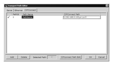
Click the **CIPCONNECT PATH EDIT** button to define the path for this application. The CIPconnect Path Editor allows the configuration of the path between your PC and the MVI56-PDPMV1 or MVI69-PDPMV1 module.
