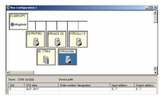
**Note:** The icon for slave 104 displays the Ident number since no GSD-file exists for this device. Also observe the configuration for the very same slave at the bottom of the screen.
