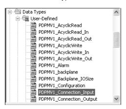
Adjust the array size for your application. The default array size is INT[250] (maximum size). This example is for 250 input words.
