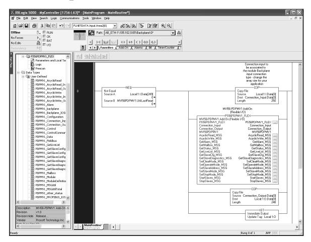
**9** The procedure has also imported new user-defined data types, controller tags, and controller tag arrays. The new Add-On Instruction can also be used through the new toolbar button (at Add-On tab).
