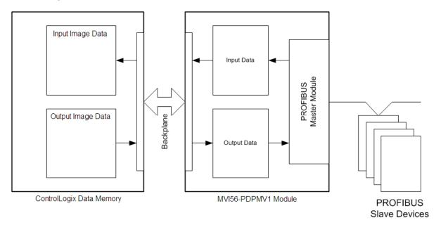
These two data blocks (Input Data and Output Data) consist of a data structure that provides for the movement of:
