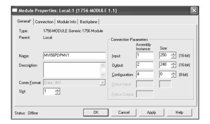
Then, the **PDPMV1\_Connection\_Input** user-defined data type must have an array size of **250** words, as shown in the following illustration.
