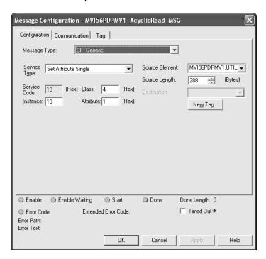
When the module has a response ready to be processed, it will latch bit 15 of the CIP Mailbox MSG Index word of the input block. The ladder logic recognizes this condition and sends another MSG instruction (now *Get Attribute Single*) to retrieve the mailbox response from the module:
