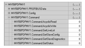
When the MSG execution is successfully completed, the controller tag MVI56PDPMV1.Util.MSG.GetStatus.DNCounter.ACC will be incremented. If an error occurs during message execution, then the controller tag MVI56PDPMV1.Util.MSG.GetStatus.ERCounter.ACC will be incremented. The error code will be stored in the controller tag MVI56PDPMV1.Util.MSG.GetStatus.LastError.
