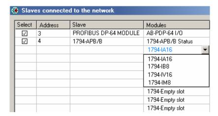
**Note**: Only modules that have the exact same Identifer bytes as the first matching module will be displayed in the drop-down list.
