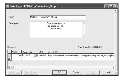
The imported ladder rung has also used the default I/O settings (Input Count = 250 words, Output Count = 248 words). If different values are used, make the following changes to the ladder logic:
