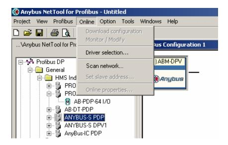
The only prerequisite for scanning the network is that the project consists of a Master with no slaves assigned to it. If a network scan is initiated and the project already contains slaves, a message window similar to the one below will appear. When the window is closed the network scan will be omitted.
