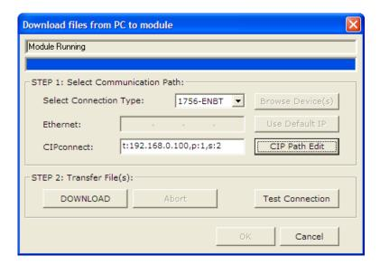
You can also monitor the PROFIBUS network through the CIPconnect path. Refer to the PROFIBUS DP section in ProSoft Configuration Builder, and verify the same path you have just created through the Download button. You can also re-edit the path through the CIP Path Edit button.
