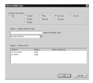
3 In the *Product Line Filter* area of the dialog box, select **MVI56**. In the *Select Module Type* dropdown list, select **MVI56-PDPMV1**, and then click **OK** to save your settings and return to the main PCB window.
