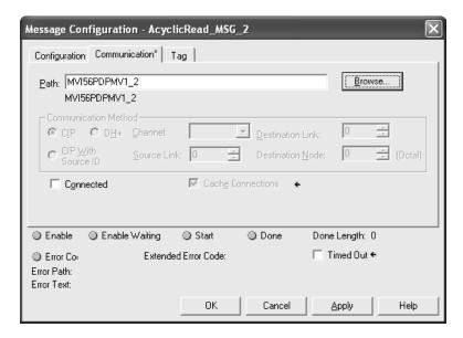
The setup procedure is now completed and the processor is ready to communicate with the MVI56-PDPMV1 module.
