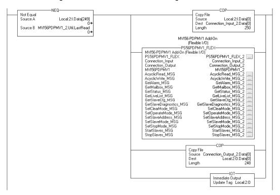
15 The module name associated with the project uses a different name than the standard "MVI56PDPMV1". You must re-define the path accordingly for each MESSAGE tag associated to the Add-On Instruction. Click the .... symbol to set up each MESSAGE tag. Select the Communication path as follows:
