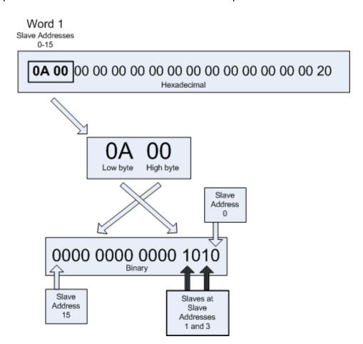
**Note:** A zero (0) in the bitmap indicates an unoccupied slave address; one (1) indicates that the slave address is occupied by a configured slave.
