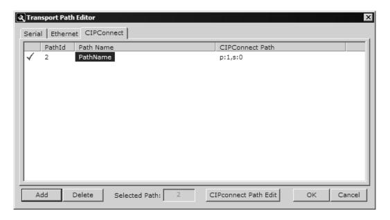
2 Configure the path as shown in the following illustration, and click CONSTRUCT CIP PATH to build the path in text format.
