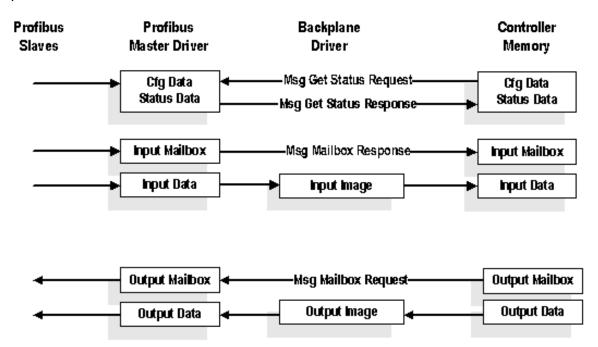
The PROFIBUS I/O data is transferred through the backplane I/O images. The status and mailbox data is transferred through MSG instructions.
