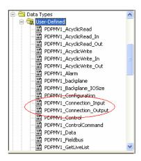
The array sizes must be modified (in the *Data Type* column) to match the connection sizes configured in the module profile. Failure to do so will prevent the module from establishing backplane communication with the ControlLogix processor.
