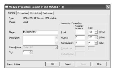
For this scenario, each backplane block reserves 100 words for PROFIBUS data, so the data fits into one backplane I/O block. The module will generate two block IDs, blocks 0 and 1, in order to force a Block ID switch, as required for the ladder logic to function correctly, but both blocks will contain the same data.
