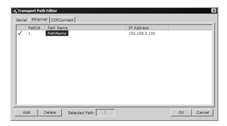
For MVI-PDPMV1 users: Select the **SERIAL** tab and enter the COM port number on your PC connected to the module. Enter a descriptive path name.
