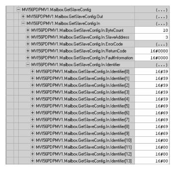
The identifier bytes will match the byte sequence displayed through PCB for PROFIBUS (*CFG data* column):
