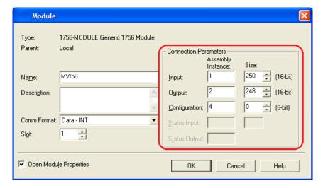
For additional details about setting connection parameters for FLEX mode, see Adjusting the Connection Sizes for Your Application (page 40).
