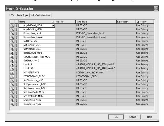
11 Change the names of all controller tags to avoid a conflict with the existing names. In this step, you should append a string to the default tag names, such as "\_2", as shown in the following illustration.
