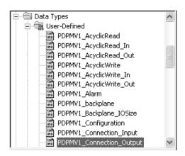
5 Adjust the array size for your application. The default array size is INT[248] (maximum size). This example is for 248 output words.
