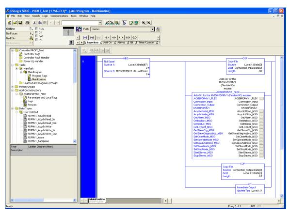
**2** Go to the *Controller Tags* window and select the **EDIT TAGS** tab. **DELETE** all the controller tags associated with the AOI import.
