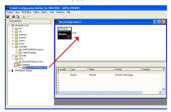
3 Drag the slave icon into the *Bus Configuration* window. This action adds the slave device and connects it to the Master in a network relationship.
