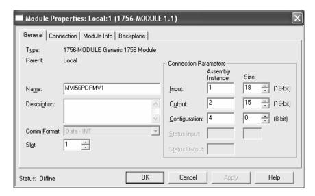
For this scenario, each backplane block reserves 10 words for PROFIBUS I/O data. The configured PROFIBUS I/O size (100 words) will not fit into one block, so ten backplane input blocks and ten backplane output blocks will be required.
