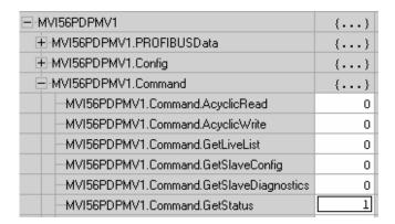
The bit is reset when the MSG instruction is enabled to request status data from the module.
