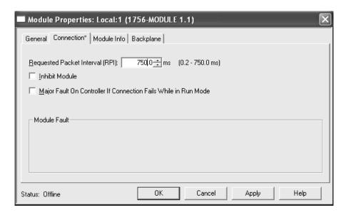
Now the MVI56-PDPMV1 module will be visible in the I/O Configuration section.
