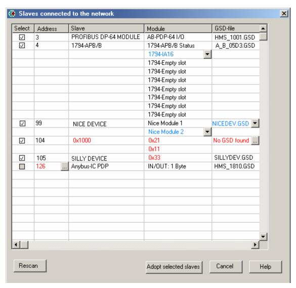
To be able to adopt a slave with address 126 the user must first assign a valid address by clicking the icon next to the node address. By doing so the Set Slave Address dialog box is started.
