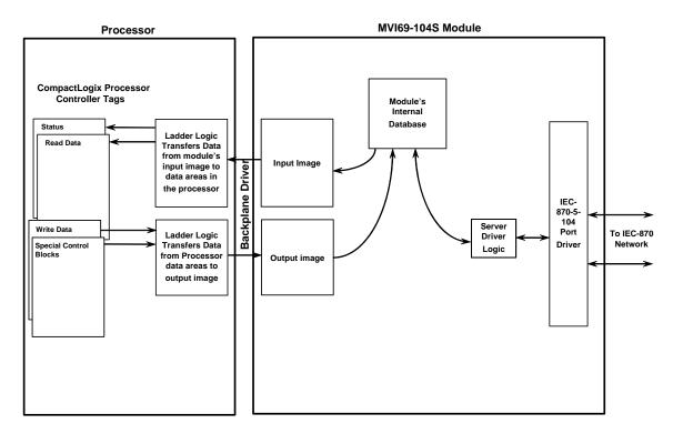
All data transferred between the module and the processor over the backplane is through the input and output images. Ladder logic must be written in the CompactLogix or MicroLogix processor to interface the input and output image data with data defined in the Controller Tags. All data used by the module is stored in its internal database. The following illustration shows the layout of the database:
