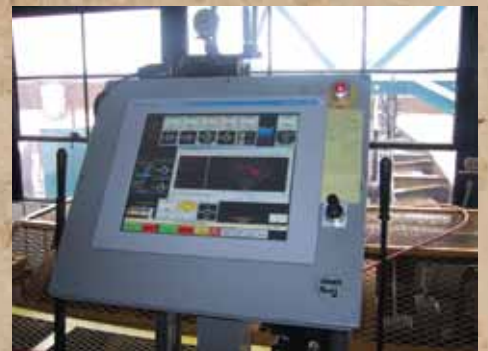
The dredge operator can watch the cutting arm via sonar on the VersaView 1700.
