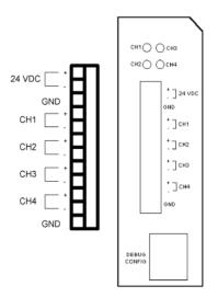
The relationship between the port labeling on the front of the module and the application is as follows:
