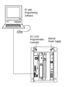
2 Connect the straight connector end of the cable to the serial port on your computer.
