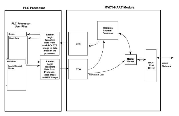
All data transferred between the module and the processor over the backplane is through the BTR and BTW blocks. Ladder logic must be written in the PLC processor to interface the block data with user data files. All data used by the module is stored in its internal database.
